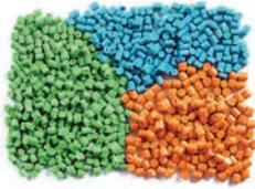
Recycled plastic is ground, melted and cooled to produce purified plastic pellets, which are tested to maintain the highest quality control standards.
